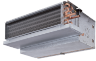
CPY - Hideaway + Plenum 200 CFM - 1200 CFM Up to 0.4" w.g. For ceiling hideaway installation
